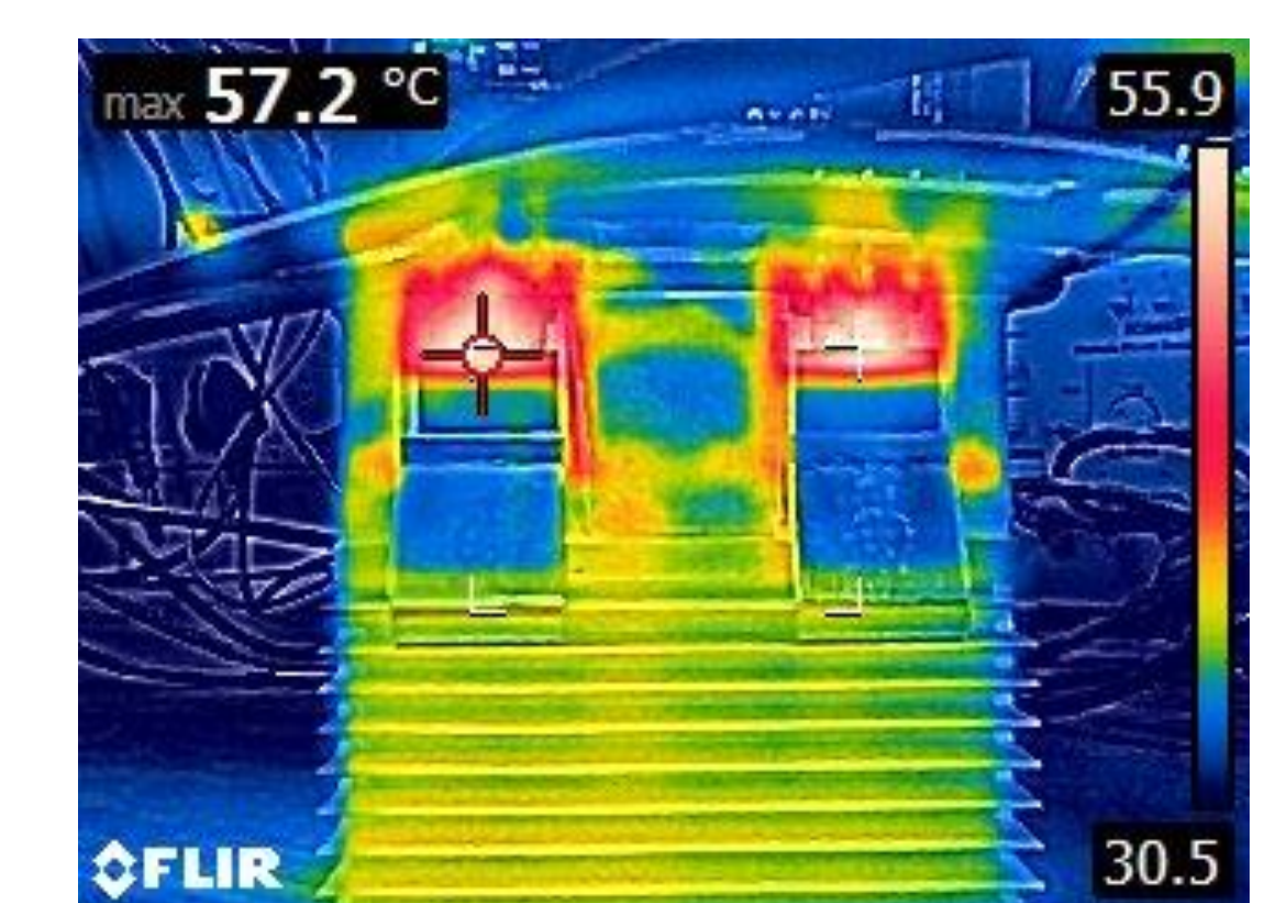
Fig. 10: Thermal image of SiC MOSFET running at 100 kHz
